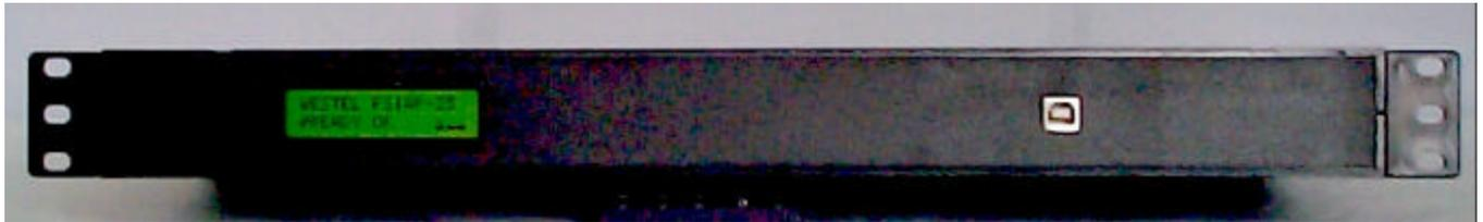
Westel's Fixed Station Interface Access Point (FSIAP-25) provides remote access and control of a P25 Base or Repeater over an ethernet network.
